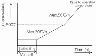
In case of lowering the temperature after dryout (for inspections inside the furnace, etc.)
