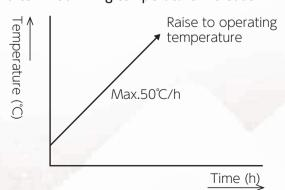
In case of lowering the temperature after dryout (for inspections inside the furnace, etc.)
