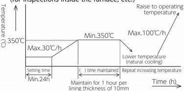
•In case of refractory lining wall with density
